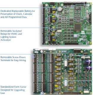
Communication Status LEDs for Transmitting and Receiving Data via RS232 / 485
