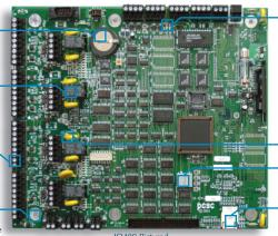
Communication Status LEDs for Transmitting and Receiving Data via RS-232 / 485
